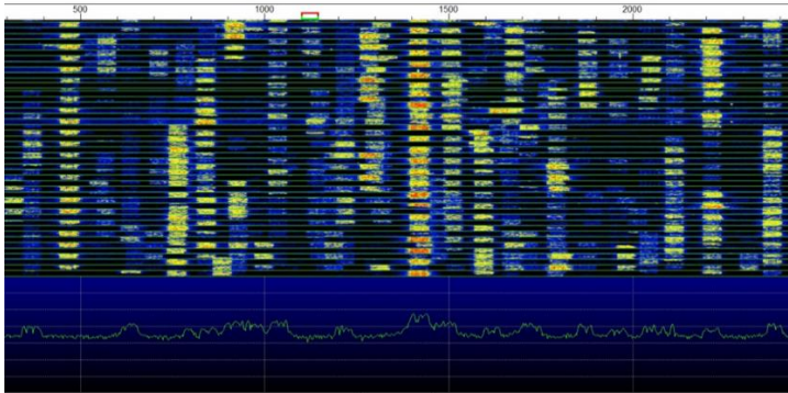
40 meter waterfall showing the popularity of FT8 – note the short 15 second intervals and faint bands near the noise floor.
