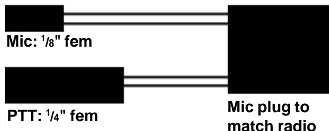
Fig. 1: Adapter: One for each radio
