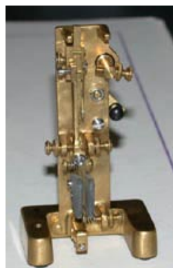
Vertical Vibroplex - 1/2-scale replica by W1KR
